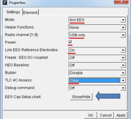
Make sure that you have selected <u>4ch EEG</u>, <u>USB only</u>, <u>Power</u> checked, <u>Link: EEG Reference Electrodes:</u> On, Click "Apply."
