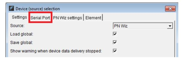
7. Select the serial port in which your PN device is connected and click "Apply". *Tip: If the Apply button doesn't appear, try resizing the Device Selection window slightly.*
