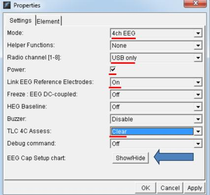
Make sure that you have selected <u>4ch EEG</u>, <u>USB only</u>, <u>Power</u> checked, <u>Link: EEG Reference Electrodes:</u> <u>On</u>, Click "Apply."
