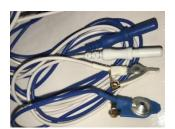
Newer caps will use long, tin ear clip electrodes that clip on the ear and plug into the amplifier (e.g. A-, B-).
