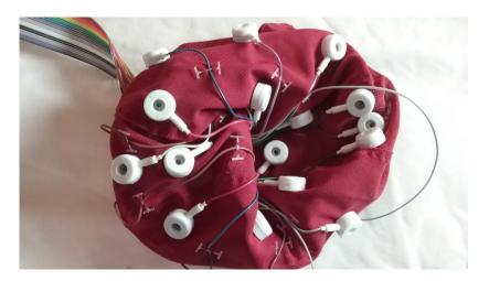
Tin electrodes are fastened into the cap and their connecting wires are tacked into it with plastic fasteners. Leave these fasteners in place. The colored wires deliver the signal to the amplifier. Please be very cautious not to stress the wires and thus disrupt the signal flowing through them.
