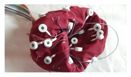
Tin electrodes are fastened into the cap and their connecting wires are tacked into it with plastic fasteners. Leave these fasteners in place. The colored wires deliver the signal to the amplifier. Please be very cautious not to stress the wires and thus disrupt the signal flowing through them.
