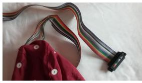
The wires from all the electrodes go from the cap to the connector end in a multicolored group. Leave these wires connected to reduce signal interference.
