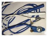
Newer caps will use long, tin ear clip electrodes that clip on the ear and plug into the amplifier (e.g. A-, B-).
