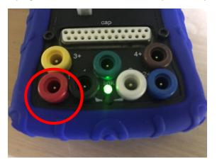
If a site is not listed, you will connect a Quick Insert electrode from the cap site to the channel port on the Q-wiz to override the cap (See "<u>Understanding default Settings</u>").
