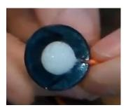
Your electrode assembly is ready for use. Before using, soak the assemblies in saline solution for a few hours so they will conduct the signal well.
